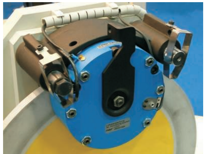
Fig. 1: The ROBA®-diskstop® is exceptionally robust and reliable. A patented alignment mechanism ensures that the brake disk runs slip-free between the friction linings during operation. The brake works with a relatively large air gap and is equipped with a highly effective patented noise-damping system which minimises switching noise even with worn linings and increased air gaps.
